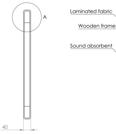
Sound absorbent DETAIL A SCALE 1:2
